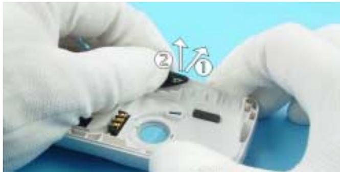
Remove Vibra Motor from its guidance.
