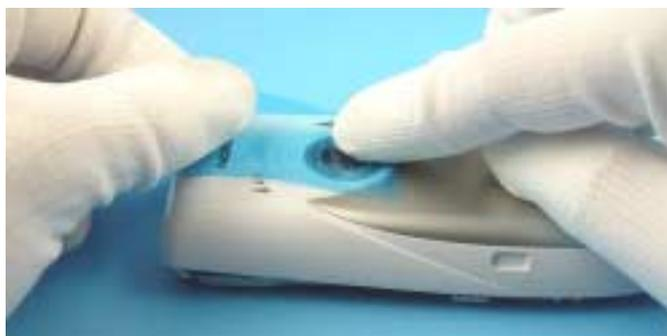
Unscrew the Torx PLUS size 6 screws using the order shown. For assembly, take reverse order and torque to 15Ncm. Always use new screws for assembly.
