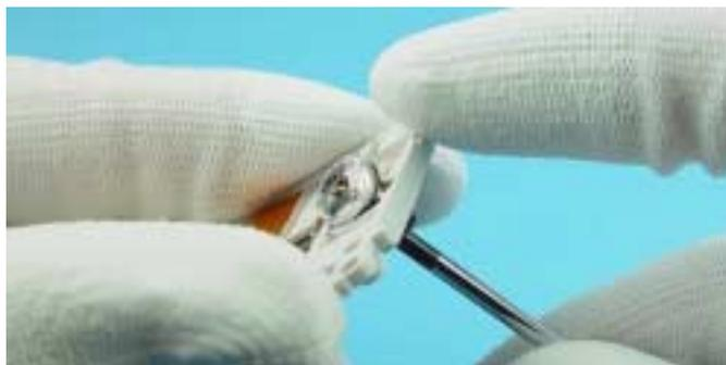
Antenna drops out when turning B-Cover.
