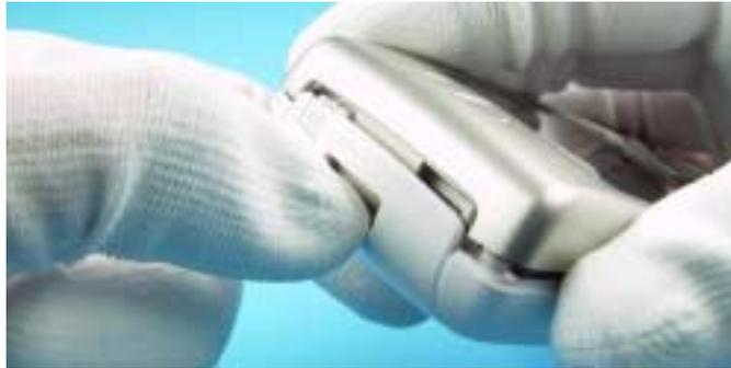
The A-Cover is attached with hooks at both sides. To remove the cover press the B-Cover carefully as shown in the picture.
