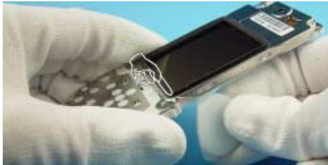
Remove the Shield and Gasket.
