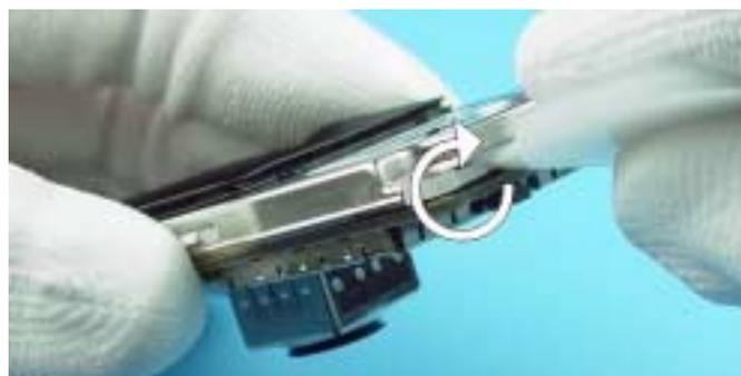
Separate LCD Module from Radio Module.
