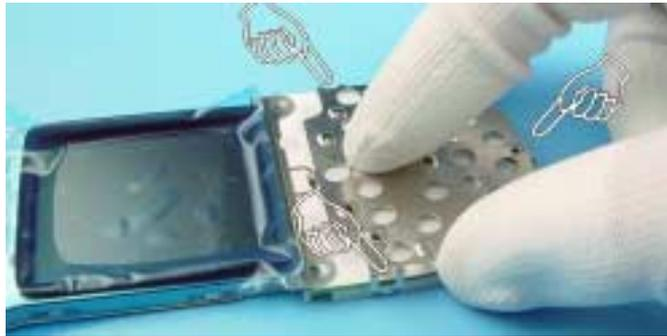
Bend UI Metal Shield latch on backside.
